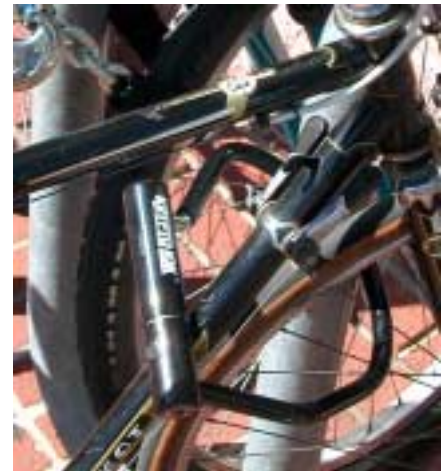
While this lock barely survived a carjacking, it is vulnerable to the dreaded BIC Pen Attack (see page 2).
